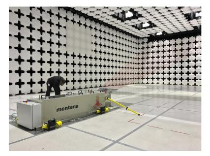
Montena's Marx generator produces a high voltage pulse, that propagates along the radiating line mounted over a conductive ground plane. The electromagnetic field pulse that is generated under the line is vertically polarised and can exceed 50 kV/m in the specified test volume. The system and the related pulse measurement equipment are controlled by software through fibre optic links. The system is designed for easy assembly and disassembly.
