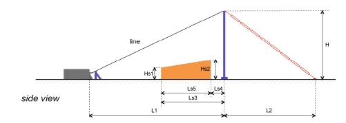
H = 50 cm $L_1 = 116 \text{ cm}$  $L_2 = 56 \text{ cm}$  $L_{s3} = 62 \text{ cm}$  $L_{\text{s4}} = 0 \text{ cm}$  $L_{s5} = 62 \text{ cm}$  $H_{s1} = 8.5 \text{ cm}$  $H_{s2} = 16.5 \text{ cm}$
