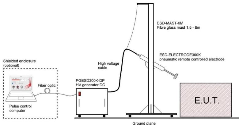
High Voltage Corona test (charged EUT) for P-static test
