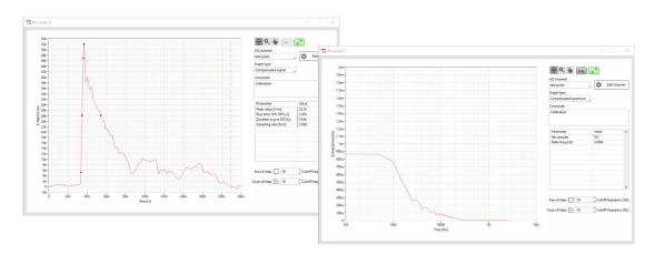
The transfer functions of all montena pulse measurement devices (sensors, baluns, fiber-optic links, ...etc) are preconfigured. The user can create and edit additional components. A more straightforward compensation approach (using constant factor and time-domain integration) can be used too.
