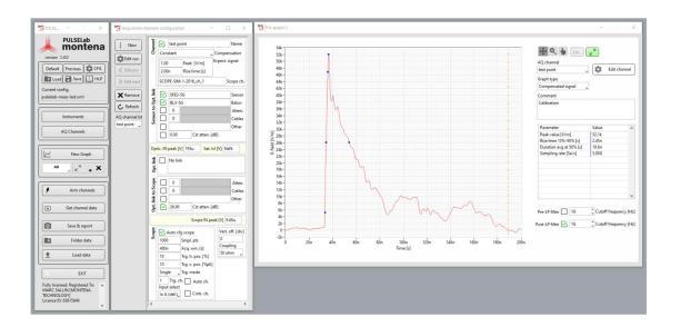
PULSELab improves the measurement accuracy by considering the transfer function of all devices used in the measurement chain (sensor, balun, attenuators, cables, fiber-optic links, etc.) and compensates the signals received by the oscilloscope to display the measured value in its own units. The correction factor of each component can be either a constant value or a frequency dependent transfer function.
