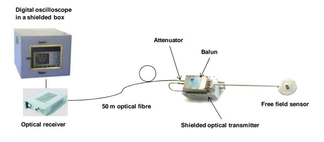
Figure 9 : free field sensor setup
