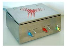
The LISN - TPD100 fulfils the MIL-STD 461 D,E and F requirements. Is consists of LISN 100 A / 270 Vac 50/60 Hz with a TPD (terminal protection device) of 100 A integrated inside the LISN and with a 20 meter shielded cable 3 x 100 A.
