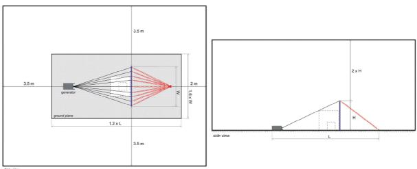
Figure 3 : minimum recommended clearance distances
