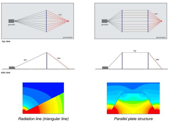
Figure 5 : triangular line vs. parallel plate structure
