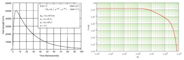
Figure 2 : MIL-STD-461E&F RS105 pulse shape and spectrum
