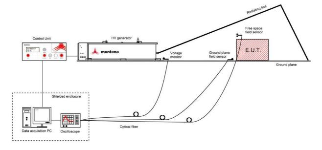
Figure 1 : schematic of a typical RS105 test setup installation
