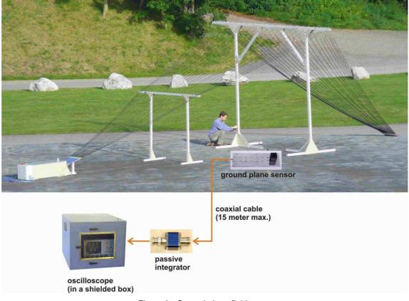
Figure 8 : Ground plane field sensor setup
