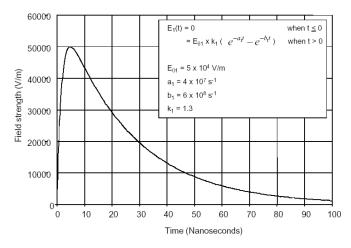
Fig. 4: figure RS105-1 of the standard - waveform of the electric field
