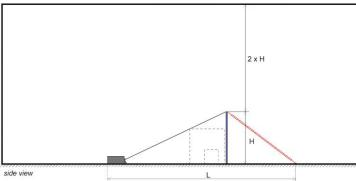
Fig. 11: minimum recommended clearance distances (for small NEMP test installations)
