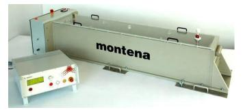
Fig. 3: Marx + peaking 360 kV NEMP pulse generator
