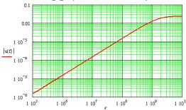
Figure 1 : Response of the sensor alone (relation output voltage / E field)
