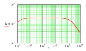
Figure 3: Response of the full system (relation output voltage / E field)
